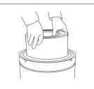
**Step 5**First remove the **HEPA filter** by placing thumbs on the inner side of the filter.
